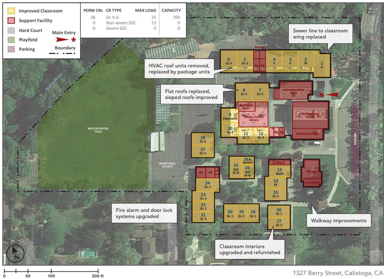
Fig. 6 – Calistoga Elementary School: Proposed Improvements
